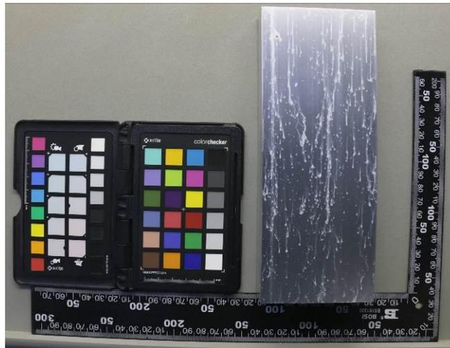
图A. 25 (AA15阳极氧化+常温封孔CASS 48h) H1
