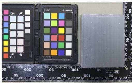
图A.15 (AA15阳极氧化+中温封孔CASS 24h) C5
