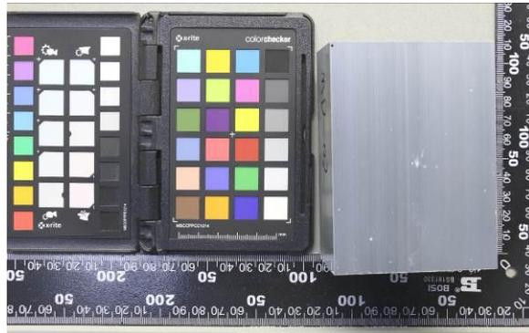
图A.12 (AA15阳极氧化+中温封孔CASS 24h) C2
