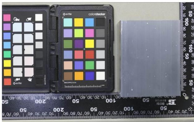
图A.20 (AA15阳极氧化+中温封孔CASS 24h) E2
