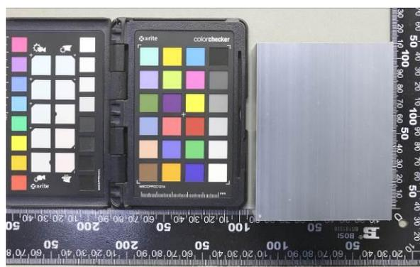
图A. 10 AA15阳极氧化+中温封孔CASS 24h B4
