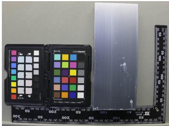
图A.21 (AA15阳极氧化+中温封孔CASS 48h) F2
