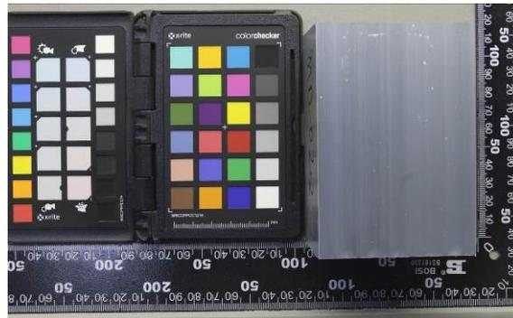
图A.13 (AA10阳极氧化+中温封孔CASS 16h) C3
