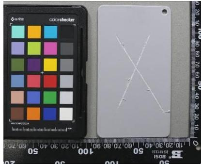
图A.63 喷粉 丝状腐蚀5mm, AASS1000h
