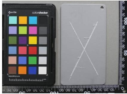
图A.62 喷粉 丝状腐蚀13mm, AASS1000h
