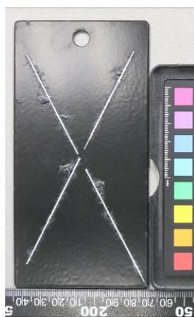
图A.54 喷粉, 鼓泡、丝状10mm, AASS1000h
